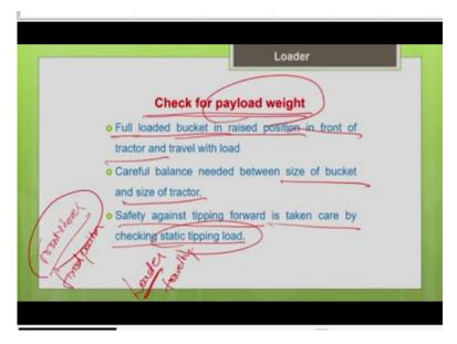
Now another important thing which we need to check particularly for the front end loaders is way to check for a payload weight from the stability point of view. So, you know that your front end loader is going to carry the material in the bucket in the front end and it has to travel for some economical haul distance. So, unlike the other excavators, which I discussed earlier, say your front shovels see if you compare this machine with your front shovel, which is also an excavator machine.
