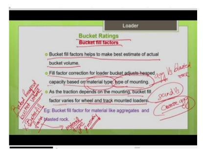
Now, let us see about the bucket ratings, see the manufacturer provide you the information on what is the heaped capacity of the bucket. So, this bucket rating is done by the manufacturer in a standard manner with a particular material, say they heap the material at a standard angle of repose say is 2 to 1 and then rate the bucket based on that. So, that bucket rating, we are going to use it for the estimation of the productivity of the loader.
