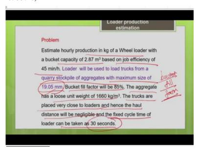
Now, let us work out the problem and see how to estimate the productivity of the loader. So, estimate the hourly production in kg of a wheel loader with a bucket capacity of 2.87 meter cube, the rated bucket capacity is given 2.87 meter cube, it is a wheel mounted loader, job
