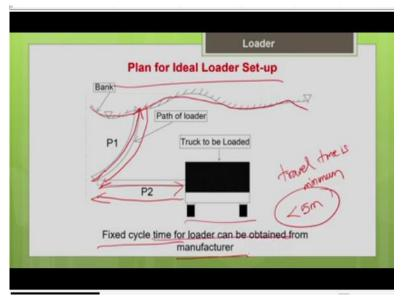
So, this picture shows the plan for the ideal loader setup. So, basically though the loader is able to transport the material for certain haul distance, it is always preferable to place the truck as close to the loader as possible particularly for the track mounted loader for which the economical distance is less than 100 meter, it is always preferable to have the truck as close as possible, so that we can improve the productivity of your loader.
