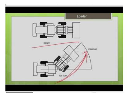
So, the machine will be in fully turn condition when they do the test. I hope you understand the difference between straight and fully turn. So, when it is fully turn it is going to be more risky. So, they carry out the test in the fully turn condition. So, basically full turn static tipping load is the loaded weight which will lift the rear wheel off the ground with the machine in static condition and fully articulated state.
