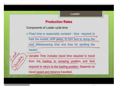
Now, let us define what is the production cycle of the loader? So, what are all the components of the production cycle as we discussed earlier the same way we can split the production cycle time into 2 components, one is fixed time, other one is variable time. The fixed time does not depend upon the haul distance, say the time needed for the loading, dumping, turning, your maneuvering the changing gears and also for spotting your truck.
