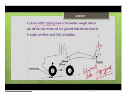
What is this tipping load? See just like you imagine you see some like if you are going to put more material into this bucket as you keep on adding material into the bucket. So, at one point of time, you can see that if the bucket is overloaded, the rear wheel will be lifted off the ground. So, that is what is called as a tipping of the bucket. So, your rear wheel will be lifted off the ground as you put more and more material into the bucket.
