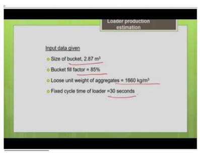
So, let me summarize the input data, size of the packet 2.87 meter cube, bucket fill factor is 85% and the loose unit weight is 1660 kg per meter cube and fixed cycle time of loaders 30 seconds.
