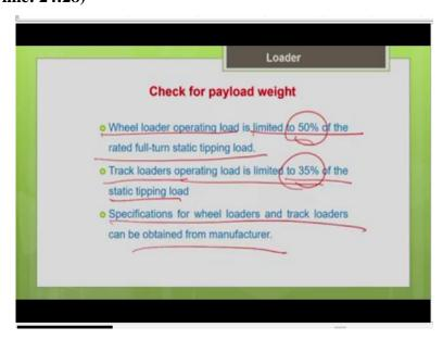
And we have to check whether the operating load of your machine that is the load in the bucket should be well within the full turn static tipping load prescribed by the manufacturer for that particular machine. So, the load in the bucket should be well within that. So, we should go for a very high factor of safety. The factor of safety depends upon the mounting of the machine.
