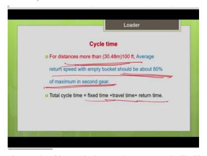
So, if the distance is more than 30 meter in that case the return speed will still more, the return speed will be for the empty bucket, it will be 80% of maximum speed in the second gear, remember when the distances are less than 30 meter, the return speed was only 60% of maximum in the second gear, but for distances greater than 30 meter, the return speed will be 80% of maximum in the second gear, it is greater for the greater haul distance. So, the total
